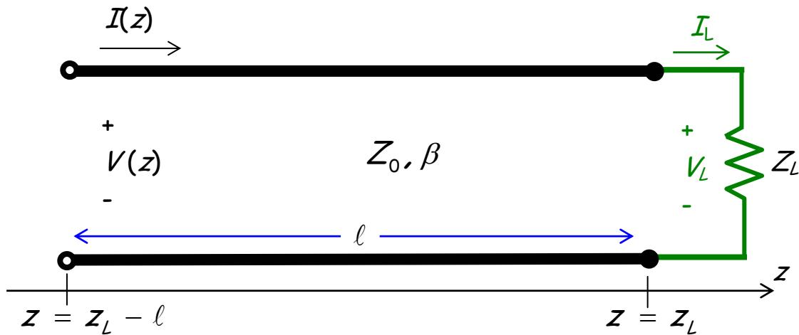
**Q:** What is the **current** and **voltage** at each and **every** point on the transmission line (i.e., what is  $I(z)$  and  $V(z)$  for all points  $z$  where  $z_L - \ell \leq z \leq z_L$ ?)?
